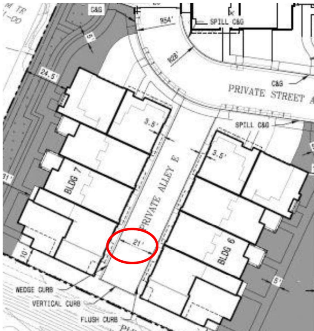
Figure 12 tight private alleys that prevent access of the emergency vehicles
