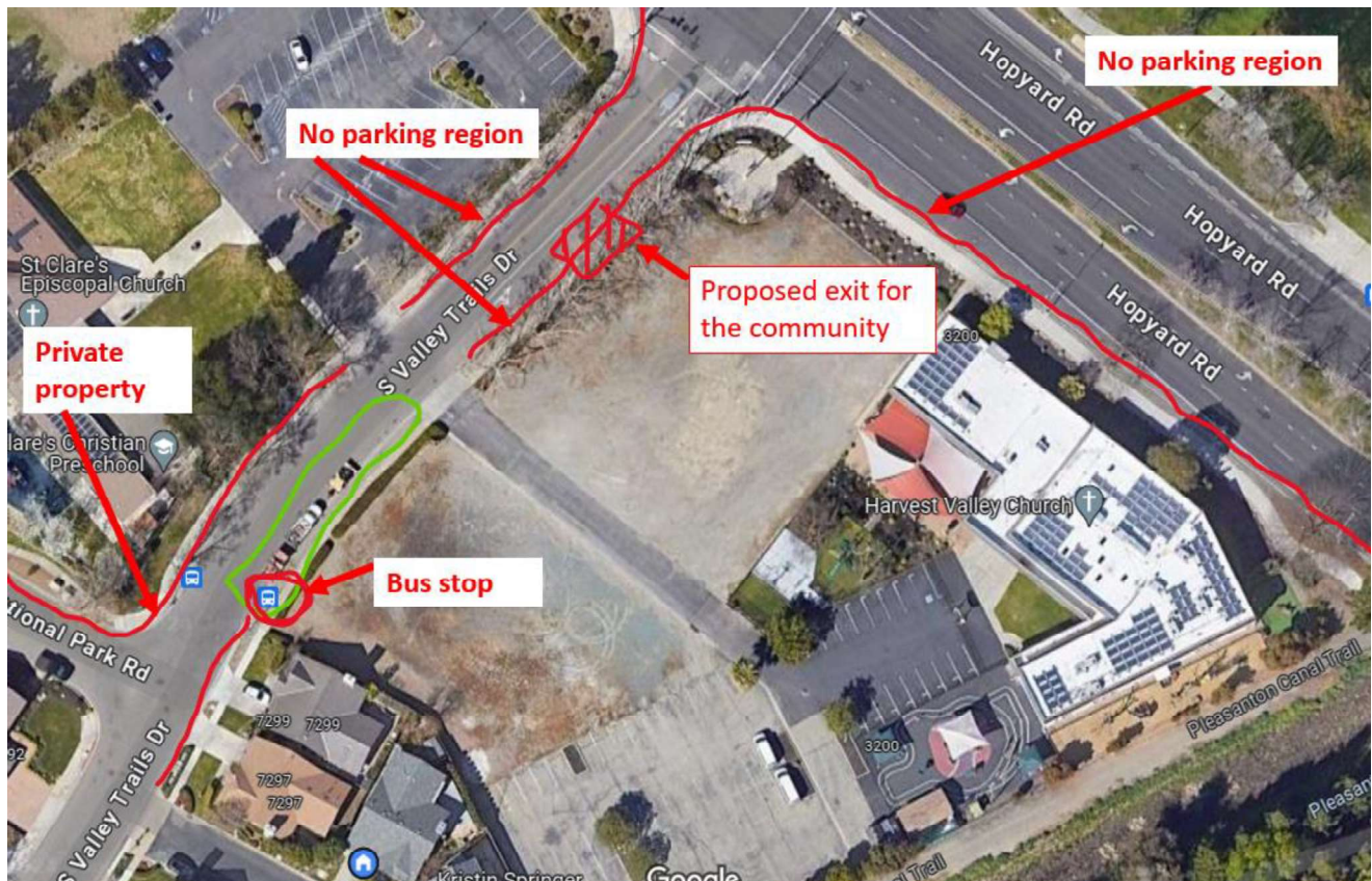
Figure 6 Major parking issues with the project: Hopyard is a main street and has no-parking policy, because of the intersection ~200ft of Valley trails is no-parking, there is a BUS STOP at a potential parking space for the lot, adding the private street close to the intersection impose major accident risks
