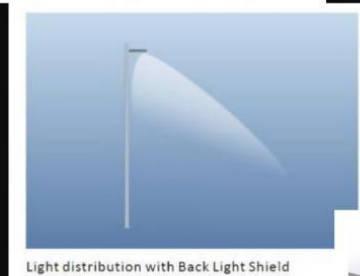
Light distribution with Back Light Shield
