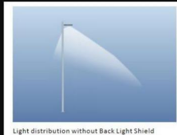
Light distribution without Back Light Shield
