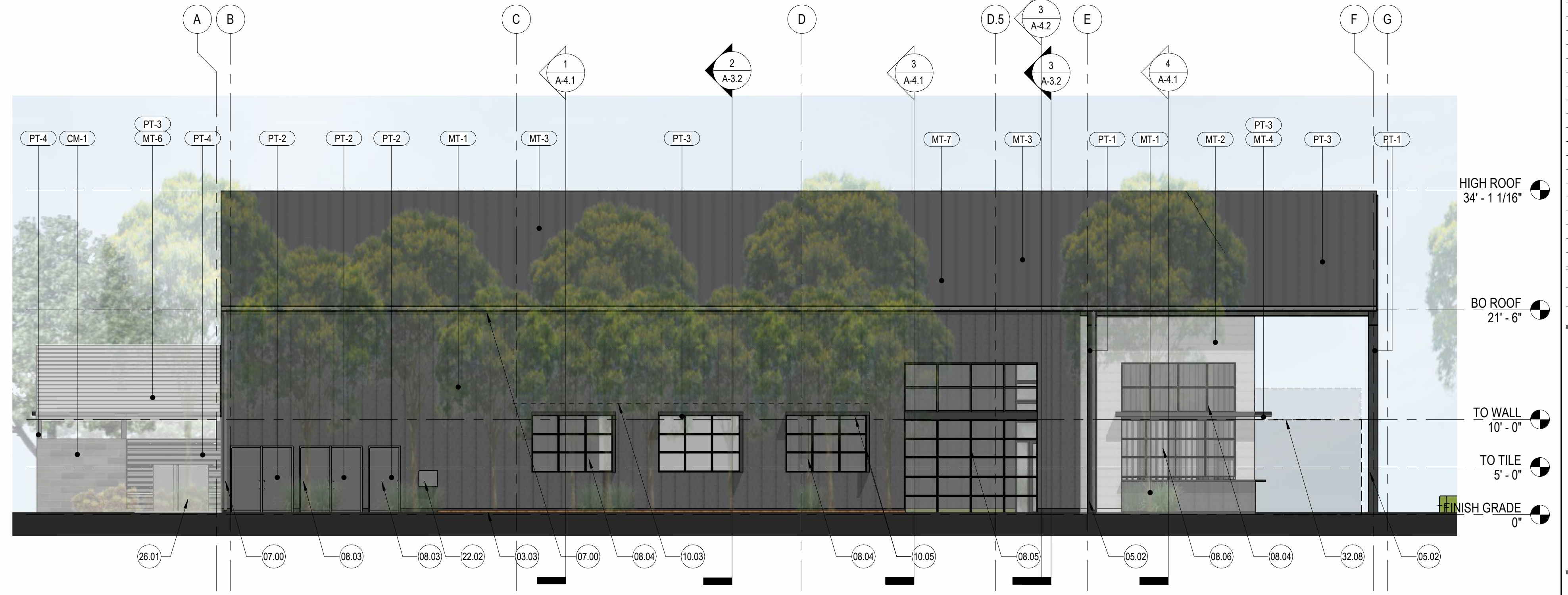
1 BUILDING ELEVATION - WEST A-3.1 1/8" = 1'-0"
